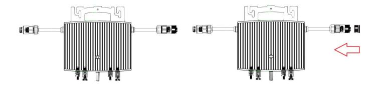
\*Note: The length of AC cable on microinverter is roughly 2 m, if the distance between two microinverters is more than 2m, please use an AC extension cable between two microinverters (as shown in the picture below).
